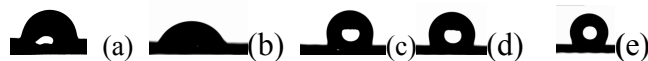
Fig. 3 Contact angles of copper-coated polyester fabrics: (a)original;(b) untreated; (c) plasma treated for 3min; (d) plasma treated for 6min; (e) plasma treated for 9min.
