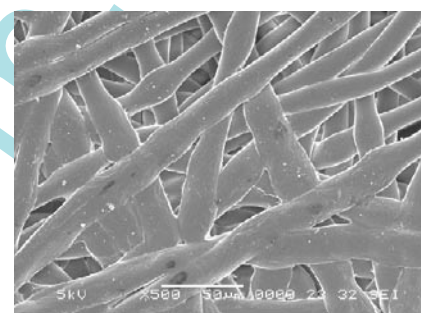
Figure 1. Untreated PET nonwoven - SEM image.
